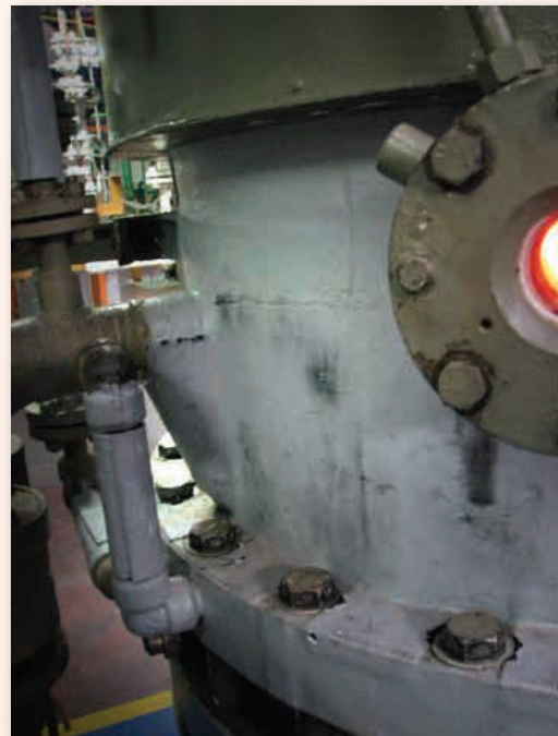
The finished surface protects the insulation during standard operations with no metallic cladding required.
